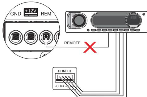
High level input must be used when the main unit does not have RCA outputs.
