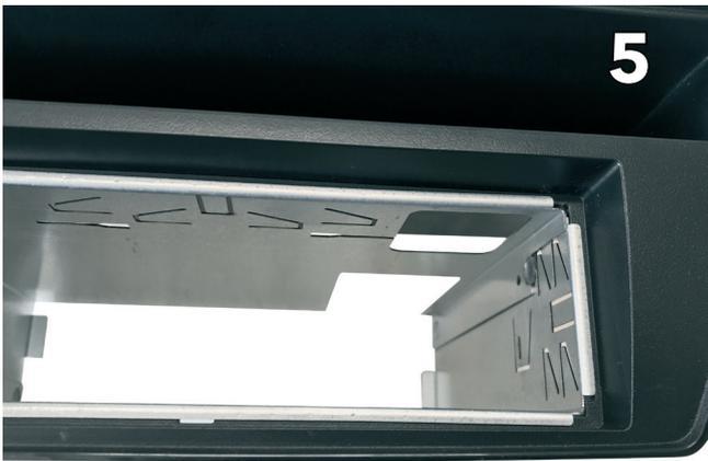
Slide the metal cage into the vehicle with the opening on top
