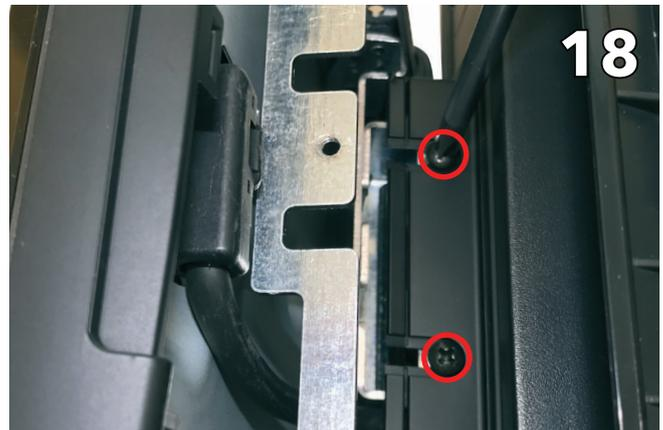
Install the neck cover onto the screen and fix the screws
