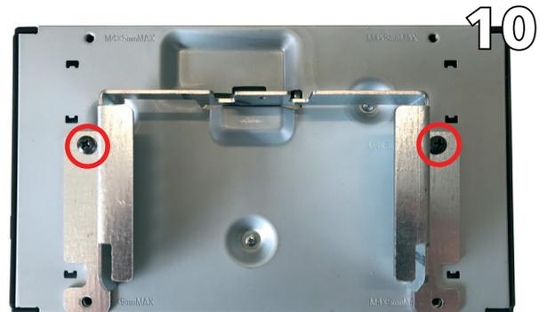
By using the two top screws, mount the screen holder to the screen
