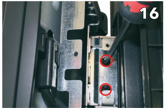
Slide the screen into the support and secure with two screws
