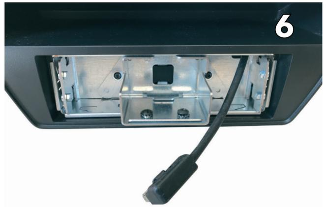
Whilst sliding the silver box in the car pull the display cable through using some tape (not included)
